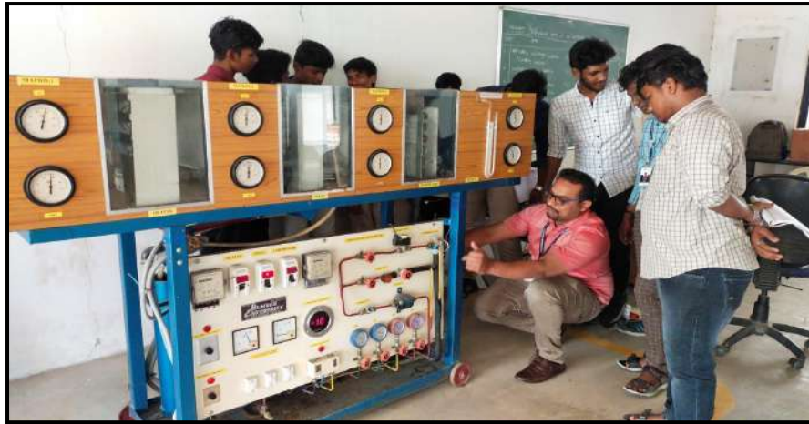
Practical session to find the performance of Air Conditioning test rig
