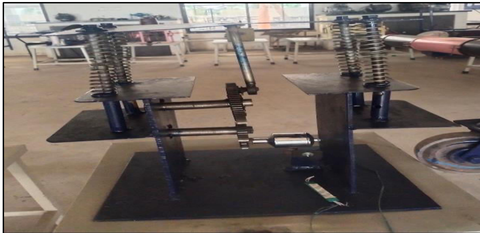
Foot Step power Generating Device
