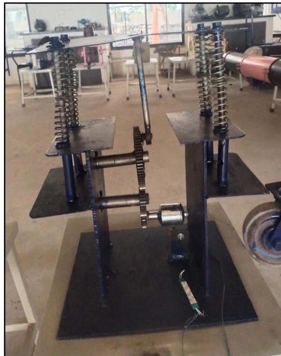
Foot Step power Generating Device
